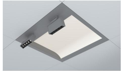
The translucent bent acrylic is purposely chosen as a reflector for indirect lighting. It absorbs and lets small amount of light travel in and out and so it softens the glare of powerful LED light. Aims non-disturbing refine light gradation on the ceiling.
