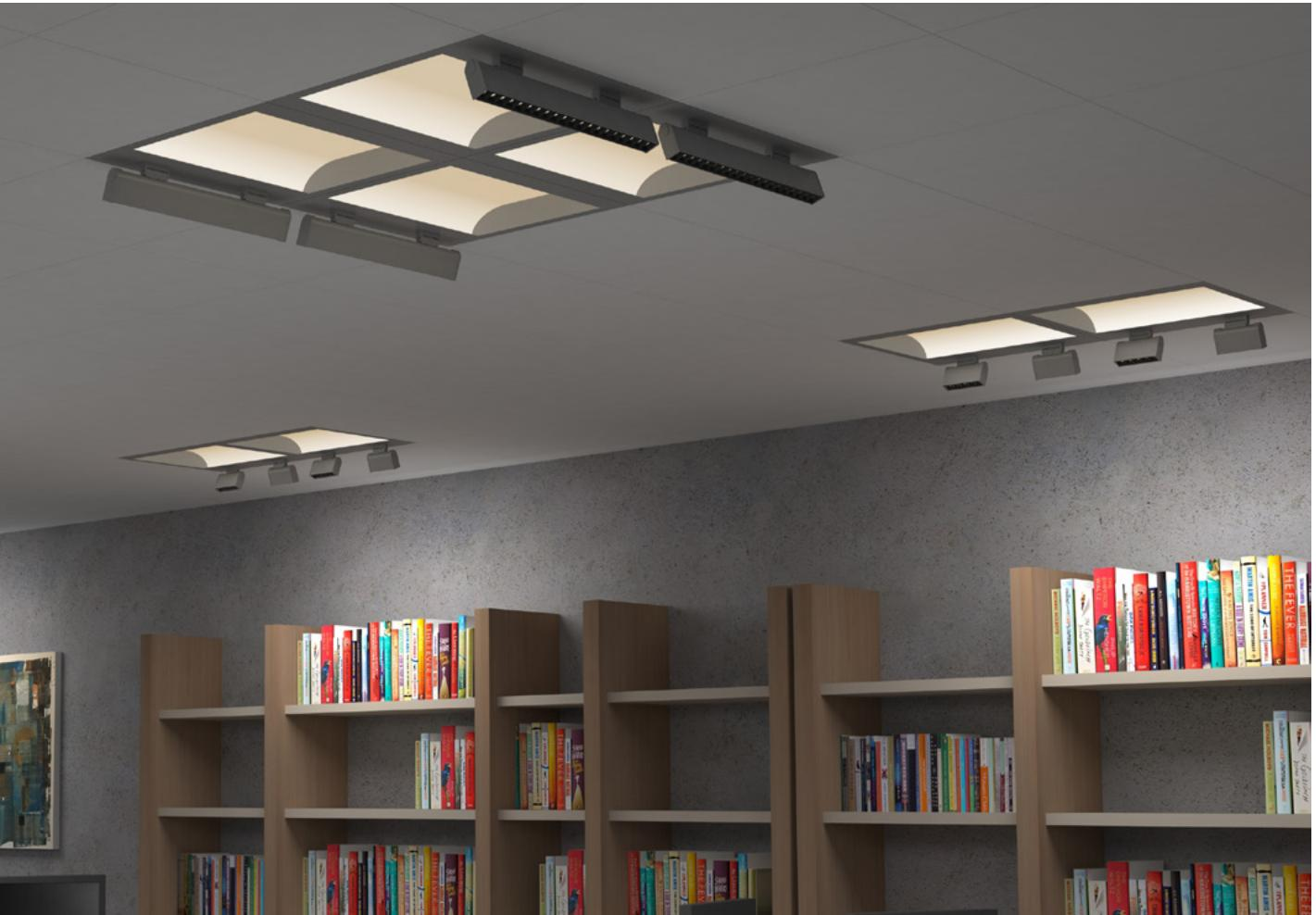
Direct lighting fixtures offer two linear-spot lights options -16 cm and 48 cm- which have slim forms thanks to compact LED light sources. They are adjustable in both direction, so are used as exhibition lighting for paintings, posters, sculptures and library lighting or as wall washer.
